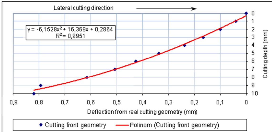
Figure 9. Characterization of cutting front geometry in the samples at 10 mm thickness.
