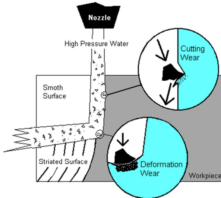
Figure 2. Kerf surface formation processes with abrasive waterjet cutting [5].
