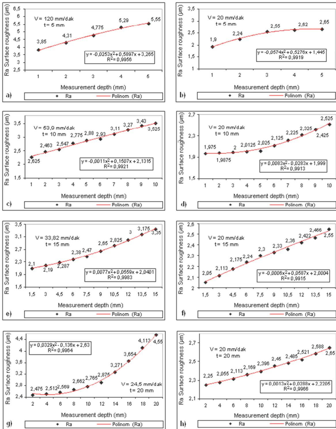
Figure 6. Parabolic (collateral polinom) models of average surface roughness values related to measurement distance that is obtained with cutting different lateral speeds of D3 cold work tool steel material in different thicknesses.
