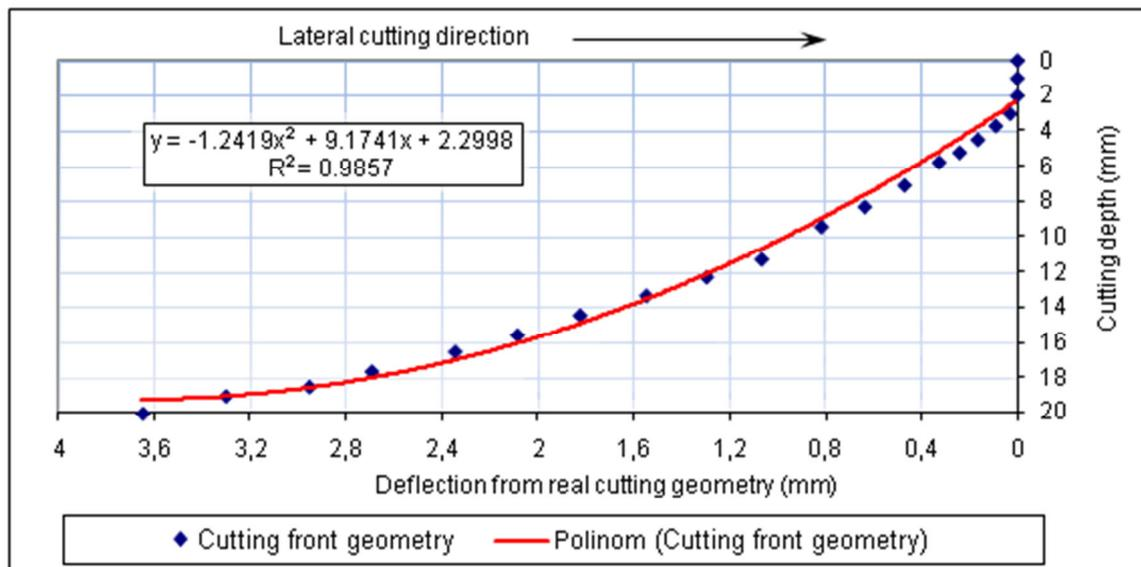
Figure 10. Characterization of cutting front geometry in the samples at 20 mm thickness.
