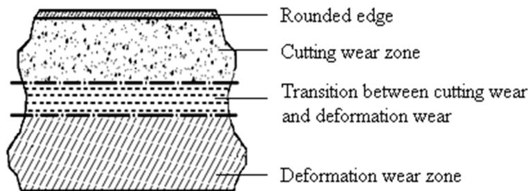
Figure 3. Surface quality that is cut with abrasive waterjet [6].
