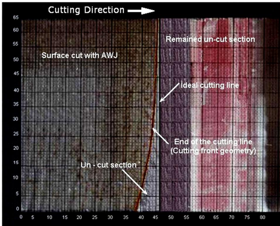
Figure 8. Determination of cutting front side geometry deviation from the ideal geometry [1, 4].
