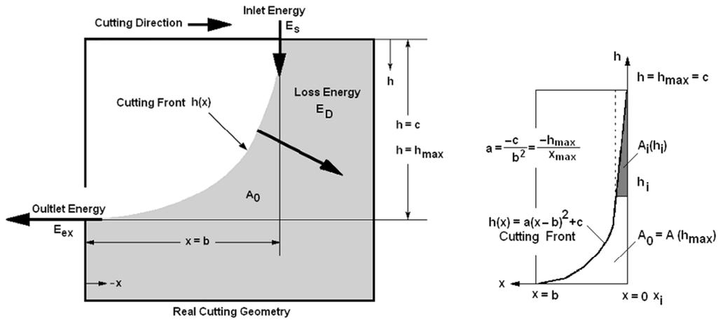
a. Formation of Cutting Front Geometry and Parabolic Model
