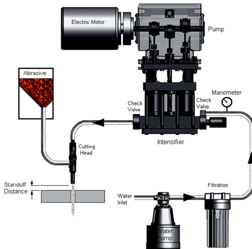
Figure 1. Schematic display of abrasive waterjet cutting system [2, 4]
