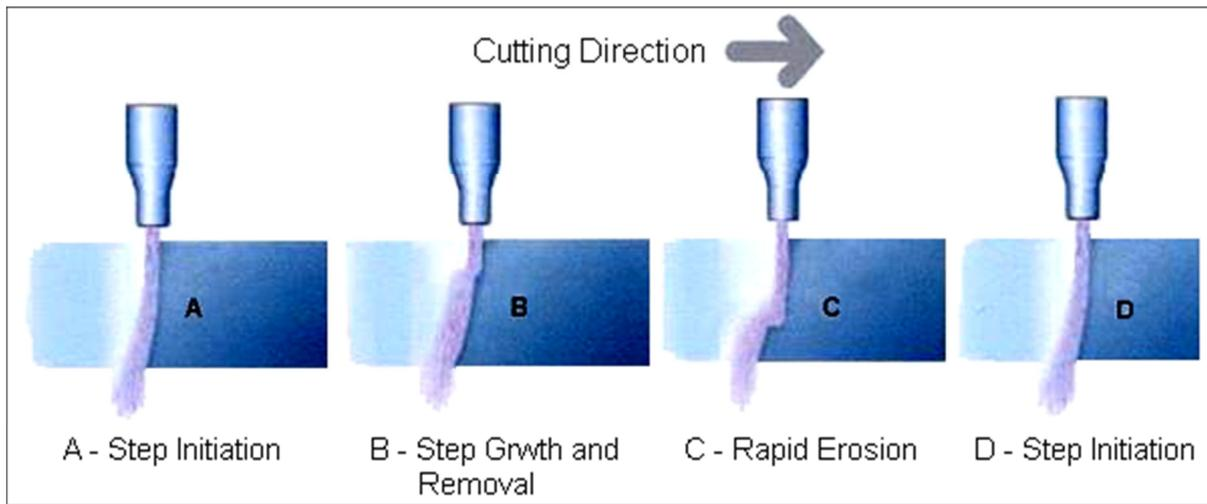
Figure 4. Formation processes of cutting front geometry [7].
