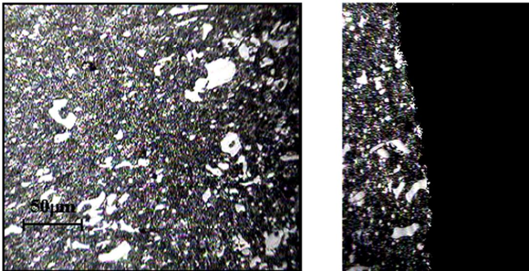
Figure 11. Micro structure of cut angle and D3 cold work tool steel material.
