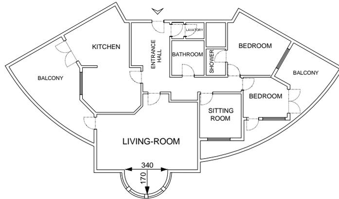
Figure 6. Typical flats of the Cagri and Acelya apartment buildings.
