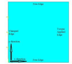
**Figure 3.** Laminated composite plates with C-F-F-F boundary conditions
