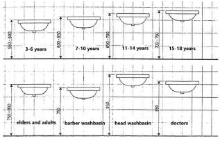
Figure 2. Standard washbasin measurements
