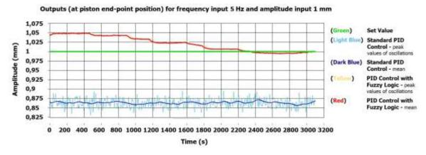
Figure 12. Comparison of output (piston end-point position) data obtained for *frequency* input 5 Hz, *amplitude* input  $\pm 1$  mm
