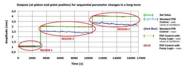
Figure 14. Comparison of output data obtained against sequential parameter changes in a long-term ( $\sim$ 300 min) test (*frequency* input 4 Hz, *amplitude* input  $\pm$ 1,  $\pm$ 3, and  $\pm$ 4 mm)
