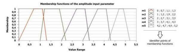
Figure 8. Membership functions and identifier points for the amplitude input parameter
