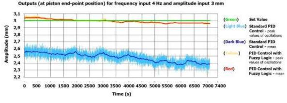
Figure 13. Comparison of output (piston end-point position) data obtained for *frequency* input 4 Hz, *amplitude* input  $\pm 3 \text{ mm}$
