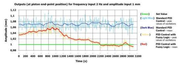
Figure 11. Comparison of output (piston end-point position) data obtained for *frequency* input 2 Hz, *amplitude* input  $\pm 1$  mm
