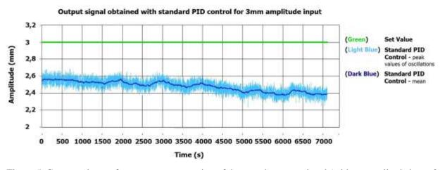
Figure 5. Comparative performance representation of the sample output signal (with an amplitude input 3 mm)
