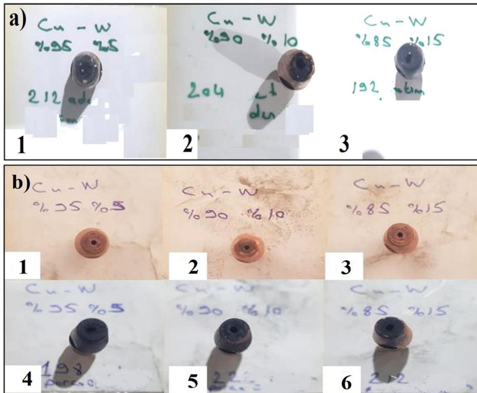
**Figure 5.** A) 1) CuW5, 2) CuW10 and 3) CuW15 contact guide images with mass production trial. B) 1) CuW5, 2) CuW10, 3) CuW15 before mass production trial, 4) CuW5, 5) CuW10 and 6) CuW15 contact guides visuals with mass production trial.
