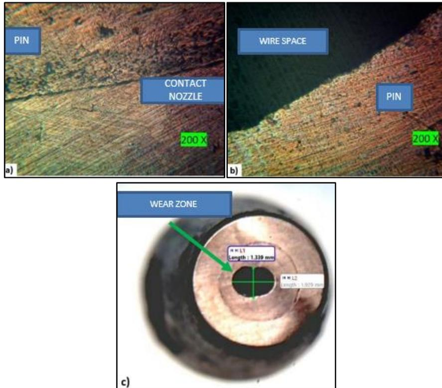
**Figure 8.** a) CuW5 microstructure image, b) Contact guide (pin) and wire feed hole 200x magnification, c) CuW5 close-up image (hole dimensions 1.929mm x 1.339mm, AR: 1.44).
