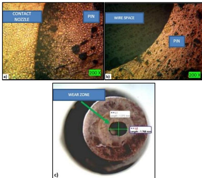
**Figure 7.** a) CuW10 microstructure image, b) Contact guide (pin) and wire feed hole 200x magnification, tested in mass production, c) CuW10 close-up image (Hole dimensions 1.768mm x 1.375mm, AR:1.28)
