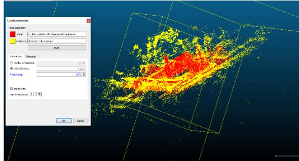
FIGURE 11. Aligning LIDAR and photogrammetry point clouds using ICP algorithm.
