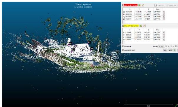
FIGURE 10. Rough alignment of LIDAR and photogrammetry point clouds.
