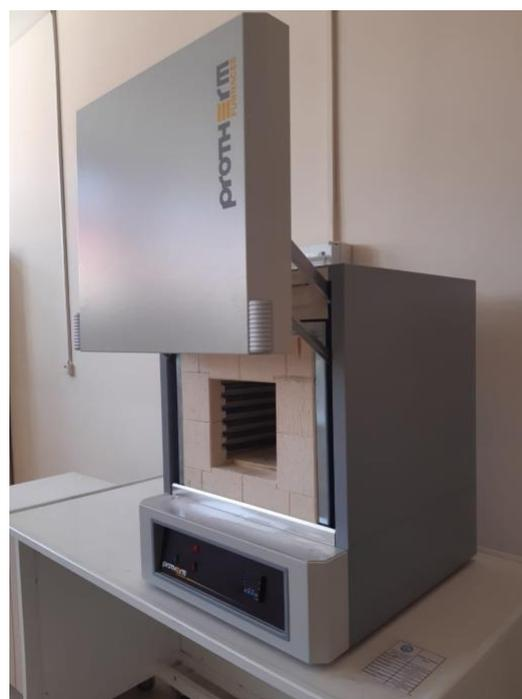
**Figure 1.** Sintering furnace.
