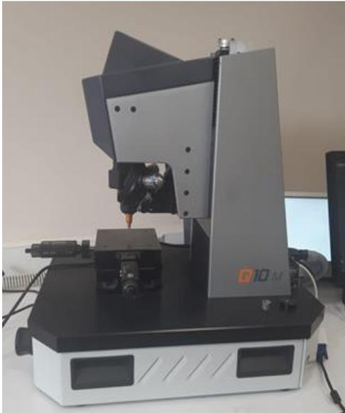
Figure 2. Microhardness tester.
