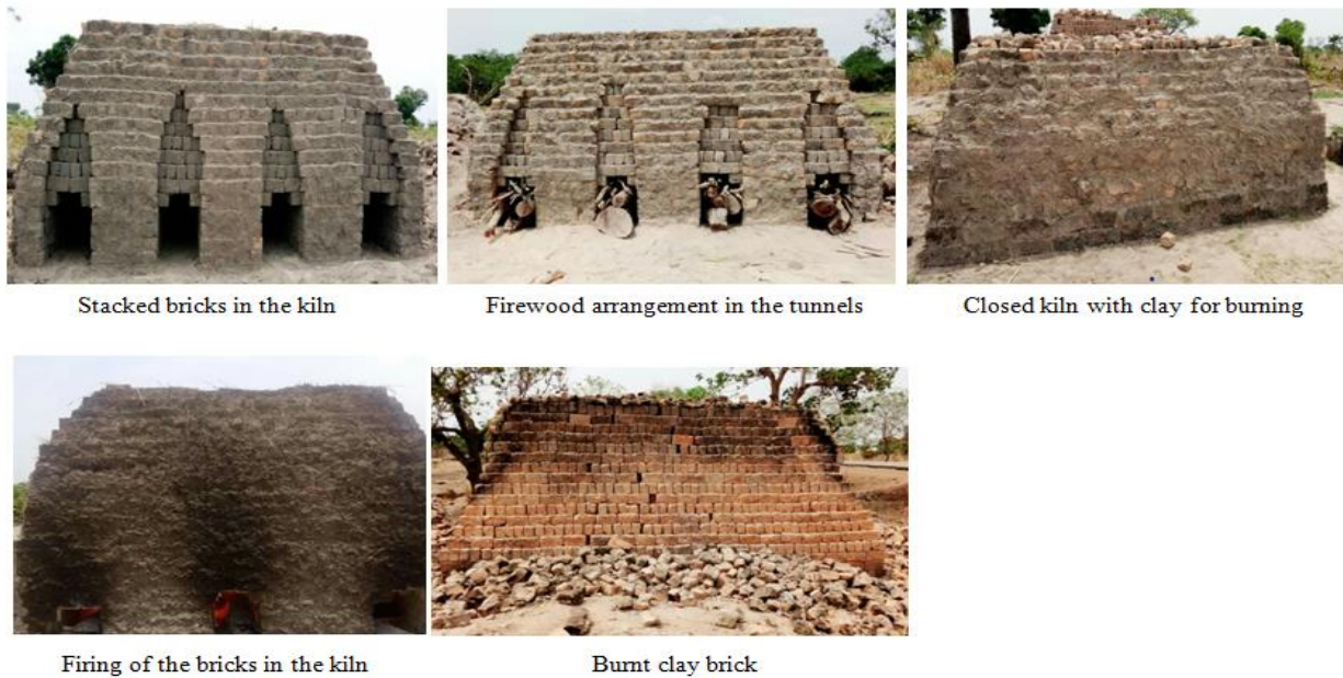
Figure 3. Firing stages in the production of bricks (field work).
