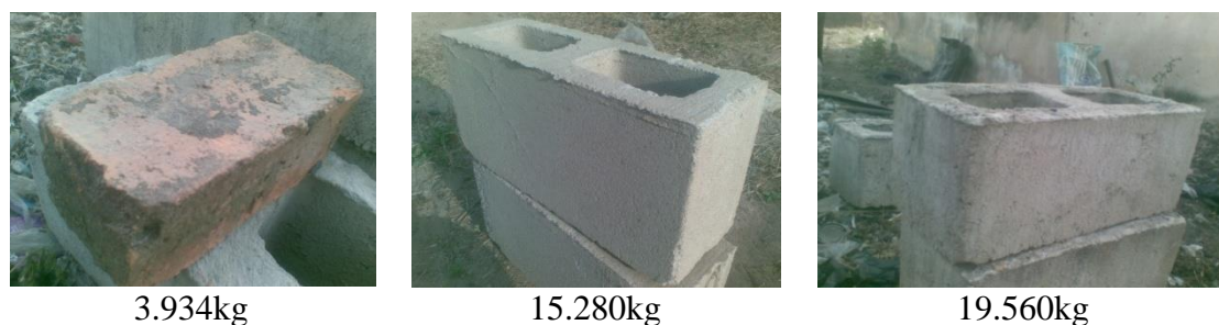
Figure 2. Building blocks used in the study
