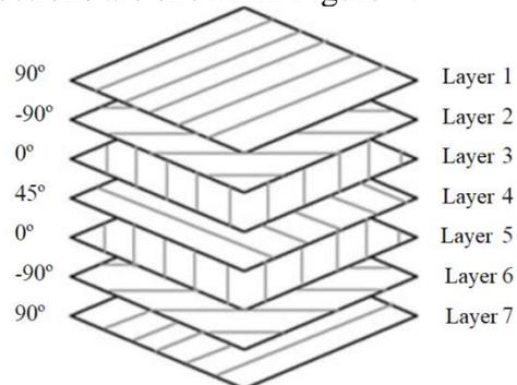
Figure 4 Composite material laying angles
