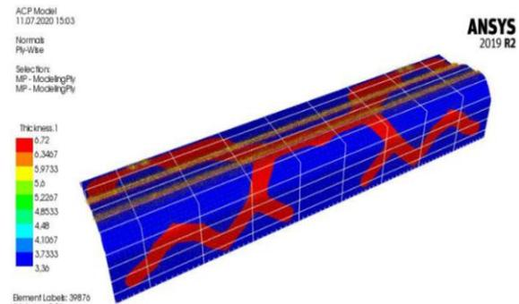
Figure 11 Final cover design with ribs added
