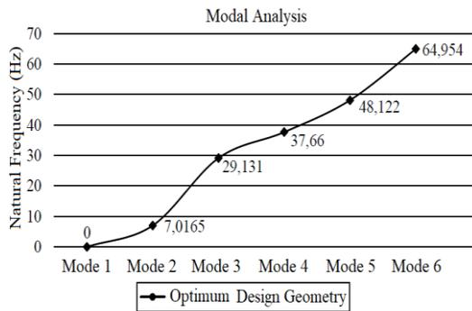
Figure 15 Modal analysis results of the valve with optimum rib geometry.
