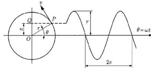
Figure 1 Simple harmonic motion
