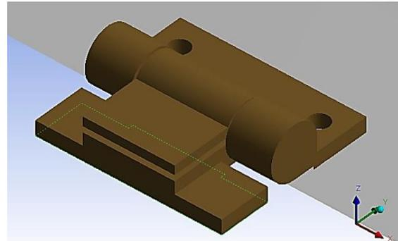
Figure 8 Fixing the fixed lug of the hinge (fixed support)
