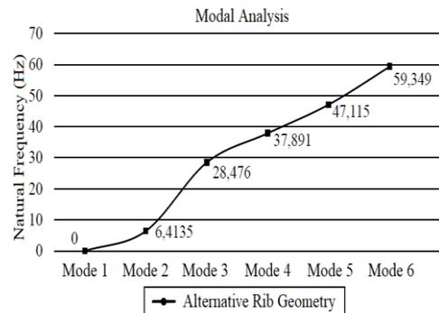
Figure 14 Alternative rib geometry modal analysis results
