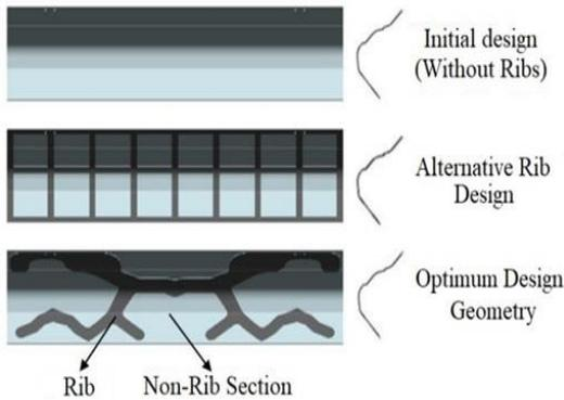
Figure 12 Initial and optimum design geometries
