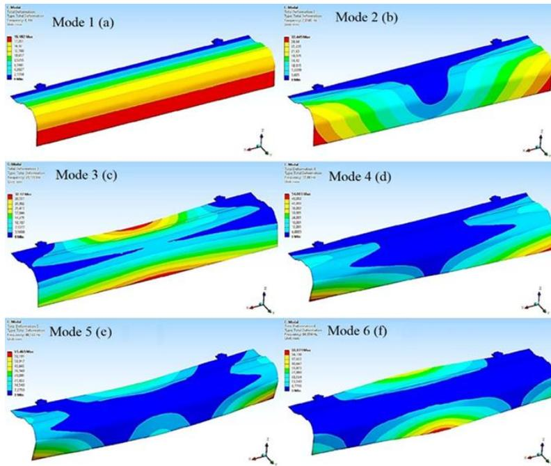
Figure 16 Modal analysis results of optimized cover design in different modes
