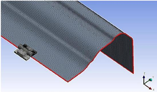
Figure 6 Finite element model of a long and flexible composite cover
