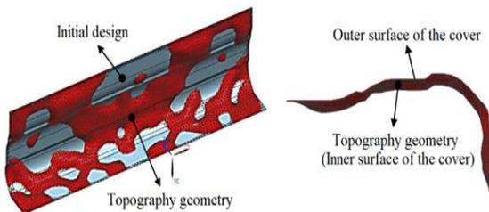
Figure 9 Rib and initial design image after optimization
