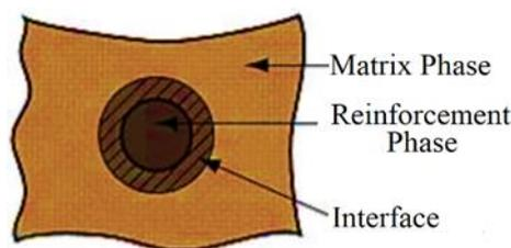
Figure 2 Composite material structure
