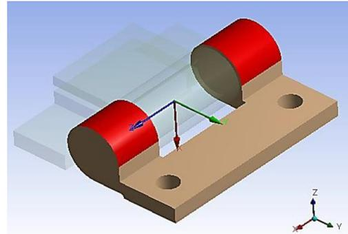
Figure 7 Hinge movable lug and door and non-moving hinge connection
