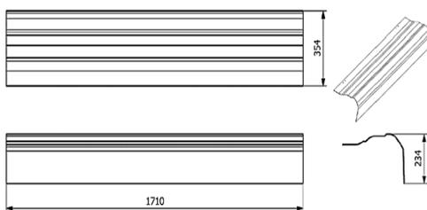
Figure 3 Long and flexible cover dimensions
