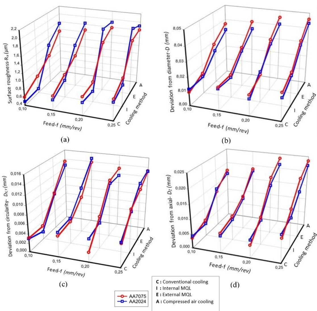
Figure 2. Variation of hole quality according to feed and cooling conditions (a): Surface roughness -Ra, (b): Deviation from diameter -D, (c): Deviation from Circularity -D<sub>X,Y</sub>, (d): Axial deviation -D<sub>Z</sub>
