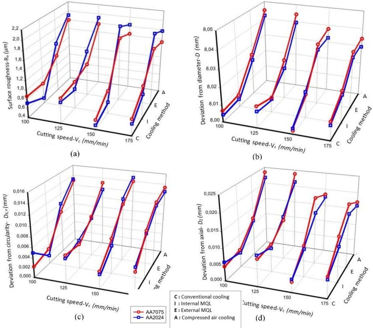
Figure 3. Variation of hole quality according to cutting speed parameters and cooling conditions (a): Surface roughness - $R_a$ , (b): Deviation from diameter - $D$ , (c): Deviation from Circularity - $D_{X,Y}$ , (d): Axial deviation - $D_Z$  (Delik kalitesinin kesme hızı parametresi ve soğutma şartlarına göre değişimi (a):Yüzey pürüzlüğü- $R_a$ , (b):Çaptan sapma- $D$ , (c):Dairesellikten sapma- $D_{X,Y}$ , (d):Eksenel sapma- $D_Z$ )
