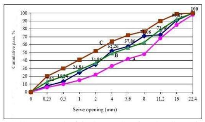
Figure 1. Aggregate granulmetric boundary curves depending on the maximum grain
