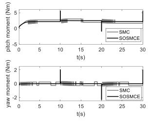
Figure 4. Pitch and yaw control signals
