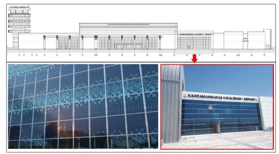
Figure 20. PV panel system installation proposal on the south facade of the existing building
