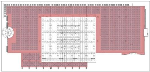
Figure 19. Suggested area for terminal building PV panel installation
