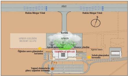
Figure 15. Terminal building layout according to bioclimatic data
