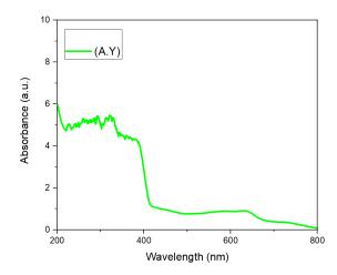
Figure 10 Absorption versus wavelength of organic green lens
