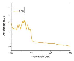
Figure 11 Absorption versus wavelength of organic brown lens
