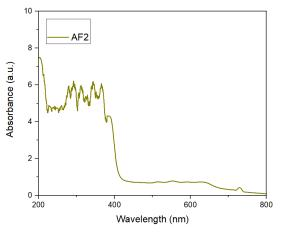
Figure 5 Absorption versus wavelength of smoked mineral lens
