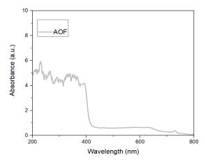
Figure 6 Absorption versus wavelength of smoked organic lens
