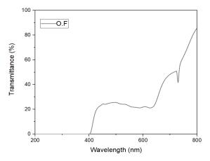
Figure 4 Light transmittance versus wavelength plot of smoked organic lens
