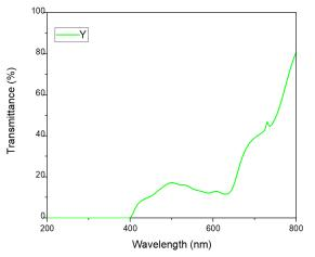
Figure 7 Light transmittance versus wavelength of organic green lens
