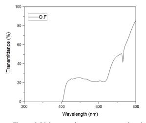
Figure 9 Light transmittance versus wavelength of organic smoked lens
