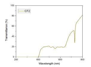
Figure 3 Wavelength versus light transmittance plot of smoked mineral lens
