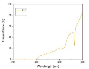
Figure 8 Light transmittance versus wavelength of organic brown lens
