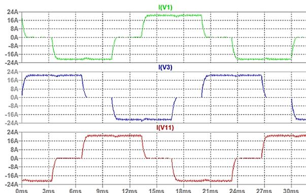
Figure 5. Phase currents A, B, C for 90% pulse width
