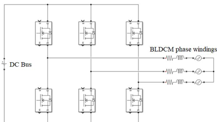
Figure 8. The Inverter Block and Motor Phase Windings
