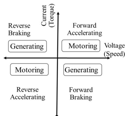
Figure 1. Quadrants of Operation Using a BLDCM [15]
