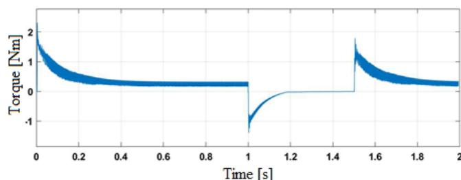
Figure 16. BLDCM Electromagnetic Torque
