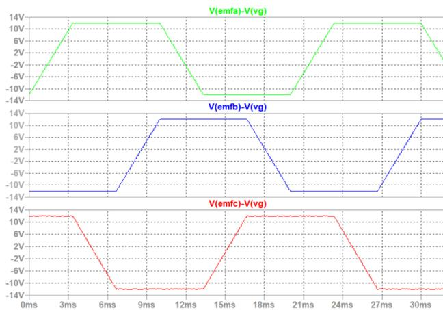
Figure 4. Back EMF voltages of phases A, B and C
