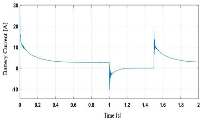
Figure 12. Battery Current of The Proposed System
