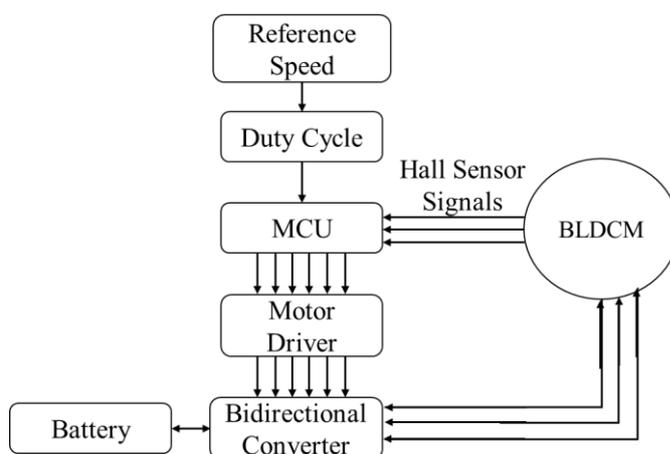
Figure 2. System Flow Diagram
