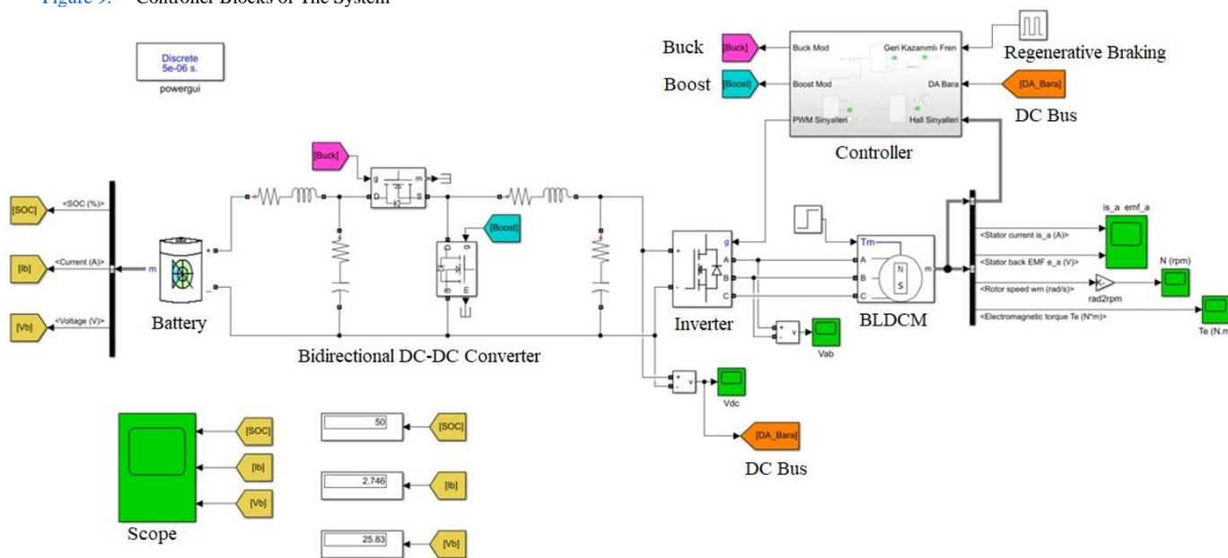
Figure 10. MATLAB/Simulink Model of The System
