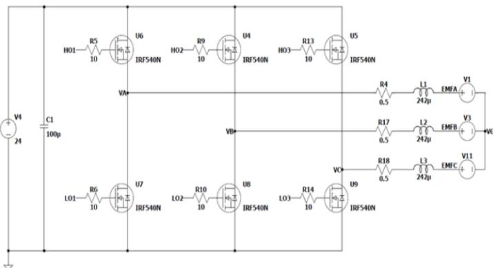
Figure 3. LTspice Model of Driver Circuit
