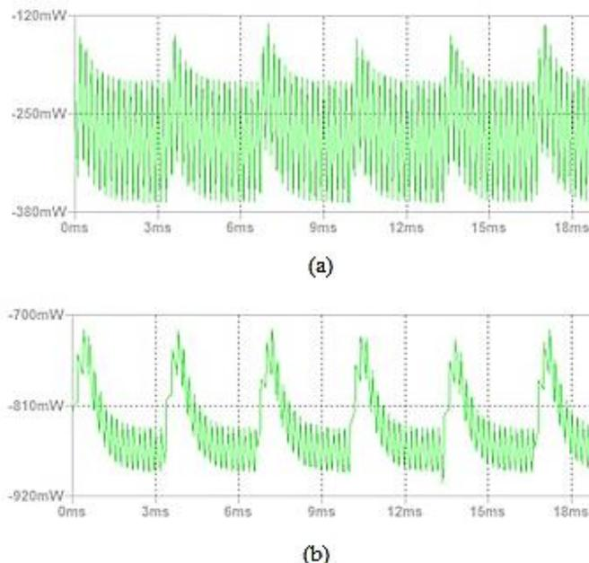
Figure 6. Electromagnetic Torque of BLDCM a) 50% pulse width b) 90% pulse width
