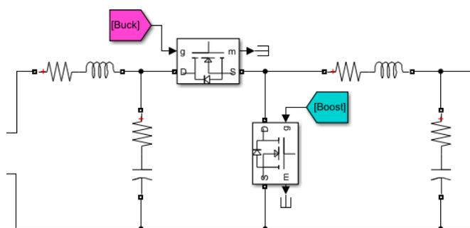
Figure 7. Bidirectional DC-to-DC Converter
