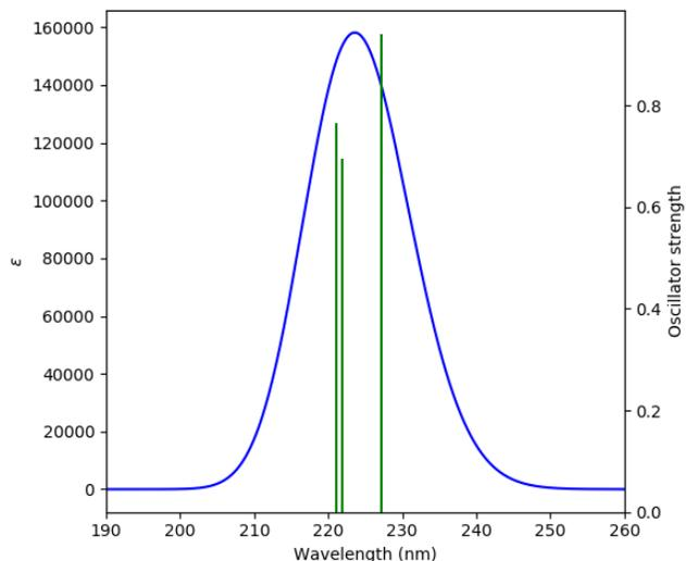
Figure 8. UV-visible absorption spectrum of Ca-Phosphosilicate
