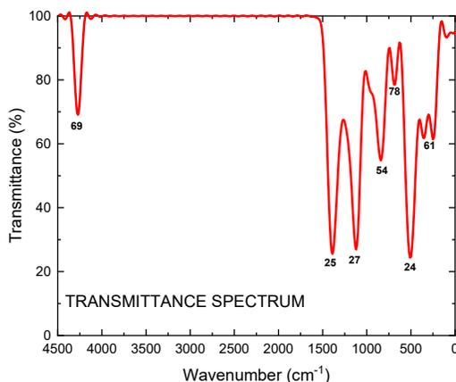
**Figure 5.** FT-IR spectrum of Ca-Phosphosilicate
