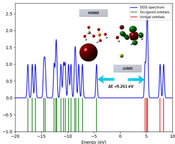
**Figure 4.** HOMO-LUMO structure with the energy level diagram and the density of states (DOS) with the contribution of Ca-Phosphosilicate
