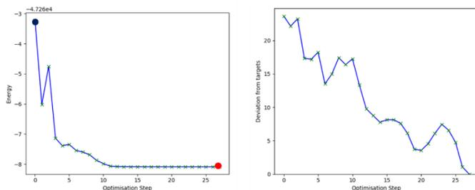
**Figure 2.** Optimization energy profile and deviation targets of Ca-Phosphosilicate
