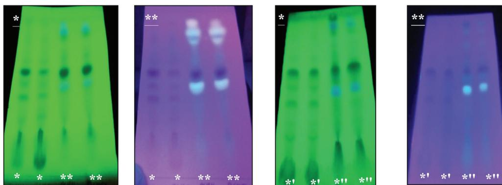
Figure 1. TLC profiles after UV revelation of the methanolic and aqueous extracts of *Z. lotus* and *R. chalepensis* harvested from Tafraoui region, in Oran (North-west Algeria). (\*) 254 nm, (\*\*) 366 nm, \*: ZL<sup>MeOH.E</sup>, \*\*: RC<sup>MeOH.E</sup>, \*!: ZL<sup>Aq.E</sup>, \*\*: RC<sup>Aq.E</sup>.
