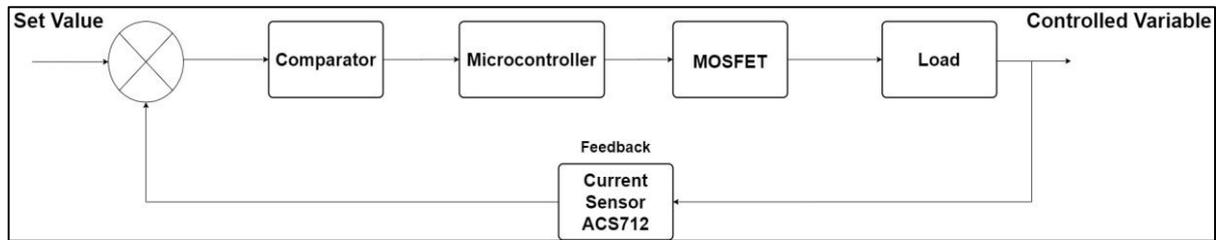
Figure 3. Block diagram of current control
