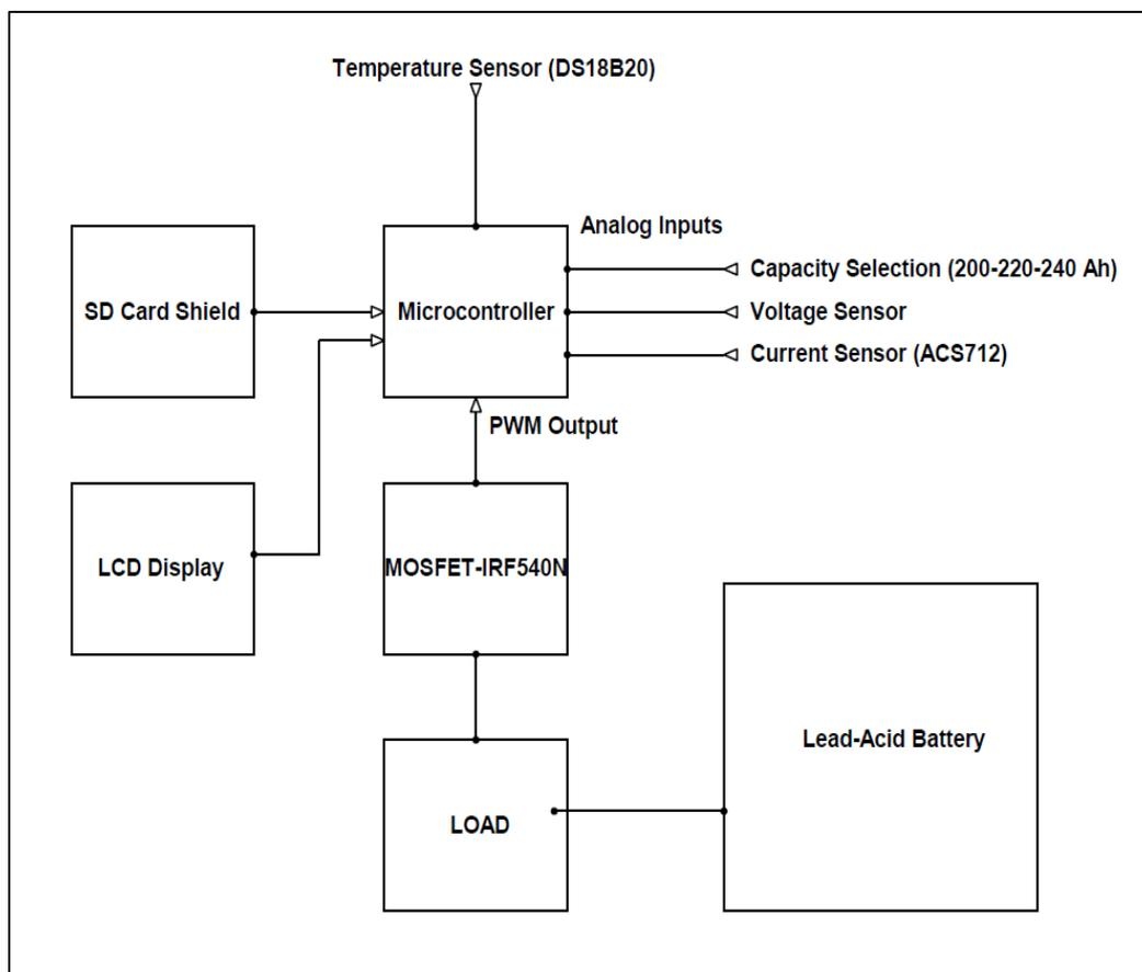
Figure 2. Hardware diagram
