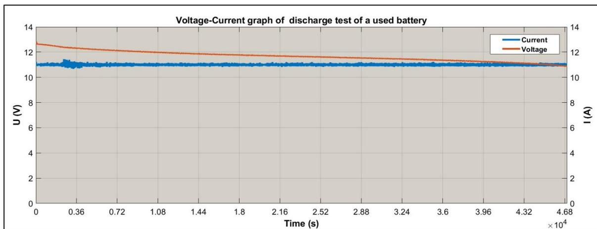
Figure 7. Voltage-Current graph of discharge test of a used battery – 220 Ah
