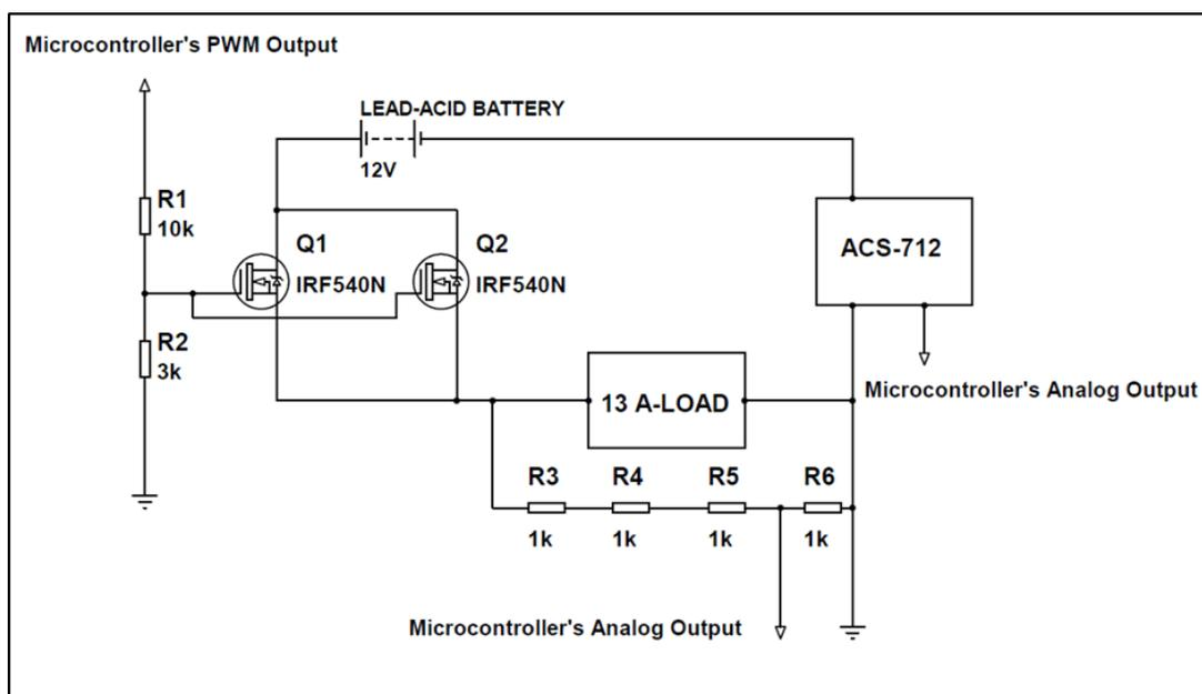
Figure 5. Battery capacity tester circuit diagram
