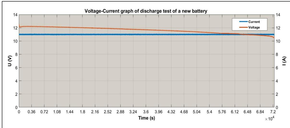
Figure 8. Voltage-Current graph of discharge test of a new battery – 220 Ah
