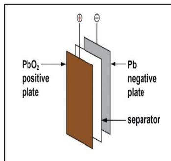
**Figure. 1. Chemistry and principal components of a lead-acid battery.**
